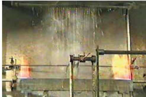
Cable then sprayed with water for 15 minutes whilst still being struck by the bar.
